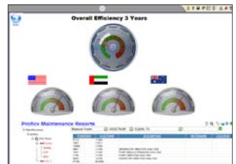
PMG Portal View: Example view showing a set of maintenance reports and equipment details that reside in the EAM system, which can be viewed in real time in the Proficiency Portal.
